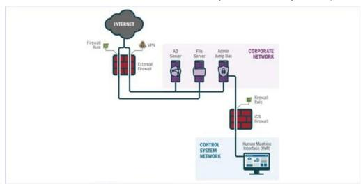
Graphic shows how Russian hackers accessed control system networks after first penetrating the corporate networks. The hackers' techniques included compromised credentials, the exfiltration of vendor reference documents from corporate servers, remote access profiles downloaded from "jump boxes" and configuration data and screenshots downloaded from human-machine interfaces. | National Cybersecurity & Communications Integration Center.
