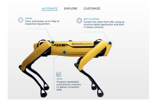
The device has a built-in thermal vision system that generates thermographic reports on the status of the different PV plant components, as it walks between the panel rows following a programmed route. According to the robot developer – US-based Boston Dynamics – the big benefit of the robot legs is that they are terrain-independent.
