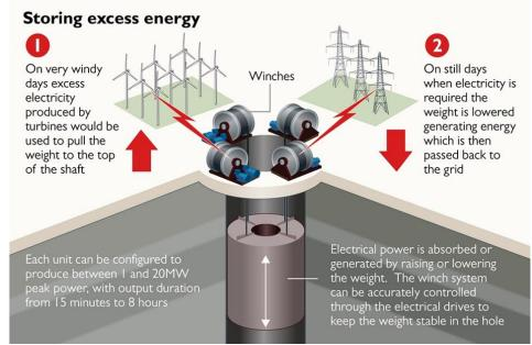
Gravitricity claims its system can operate for up to 50 years and store energy at half the cost of lithium-ion batteries. In India, it has partnered with Panitek Power on the 12month project, which aims to identify and shortlist sites for a demonstration scheme. Gravity storage is a relatively simple technology. It doesn't rely on any rare earth metals, and has a very long lifespan, so it can be manufactured and deployed locally, said Chris Yendell, project development manager at Gravitricity.
