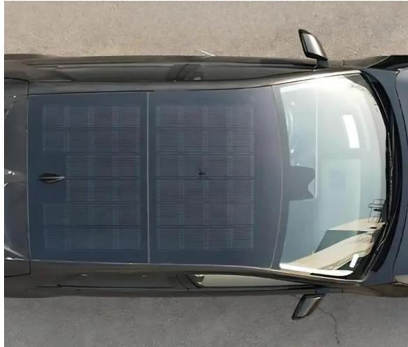
“Traditionally, solar panels for cars are made with glass, but glass is heavy and limits vehicle design. Our solution uses polymer packaging, which is much lighter and allows for more flexible vehicle designs.”
